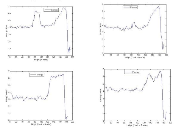
Plot of entropy vs height for fog formation and dispersion stages (top 2 plots) and fog formed stages (bottom 2 plots)
