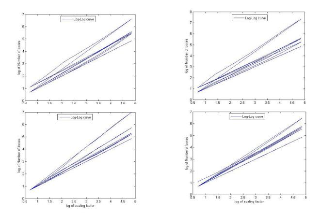
Plot of log (boxcount) vs log (scale factor) for fog formation and dispersion stages (top 2 plots) and fog formed stages (bottom 2 plots)
