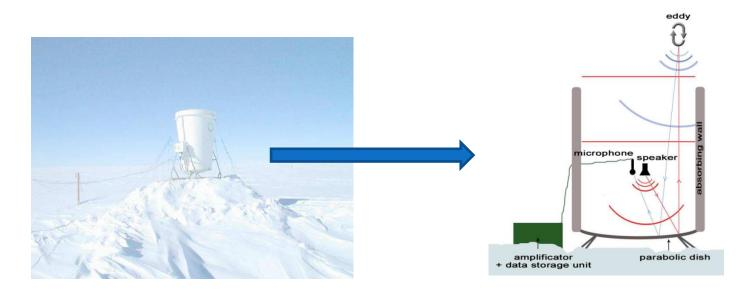
**SO**nic **D**etection **A**nd **R**anging also known as **SODAR** is very efficient way to explore the time evolution of lower atmosphere. Acoustic pulses of short duration are transmitted upwards using an acoustic antenna. These pulses gets refracted and backscattered due to temperature inhomogeneity and gets recorded in SODAR. (pictures taken from website of Halley British Antarctic Survey)
